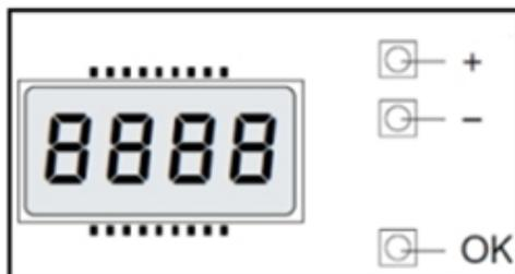
1. Press the "OK" button on your receiver twice. The screen displays "PARA."
